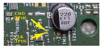
Figure 7: ISP points for Echo Dot 3rd Gen on PCB back side
